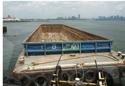
Beginning the turn. The boat is angling off to starboard and pushing the bow around to port, as well as, ahead.
